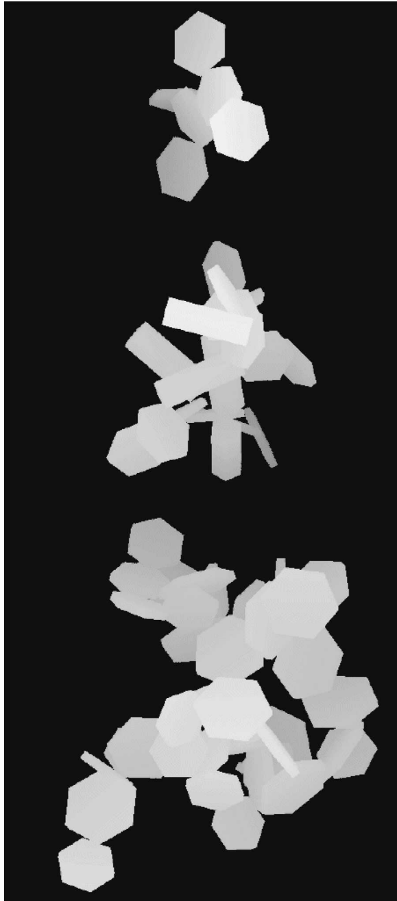
FIG. B2. Some Z-buffer images showing one particle from each of the three sets of random hexagonal aggregates. (top) An aggregate of 6 of the thinner plates, (middle) an aggregate of 20 plates and columns, and (bottom) an aggregate of 40 thicker plates. The lighter shades indicate the closer parts of the particle, and the darker shades indicate the farther parts.
