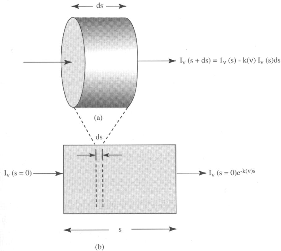
(a) Intensity passing through a thin slab suffers extinction proportional to the path length  $ds$ .
