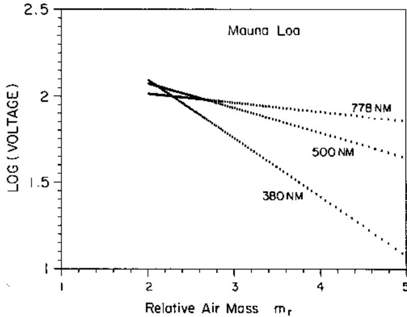
An example of a Langley plot for three wavelengths showing Sun photometer log voltage vs. air mass ( $\sec \theta_0$ ) for clear conditions. [Stephens, 1994, Fig. 6.1]
